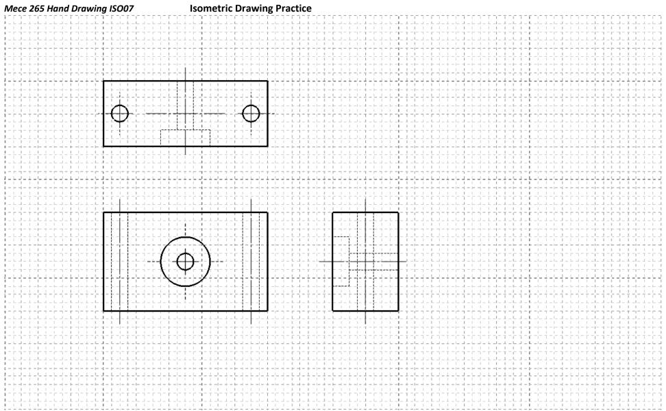
**Connecting Block: Draw the Isometric View**
